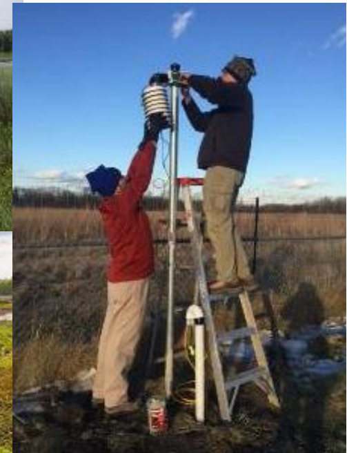
Waggle/AOT node deployment
