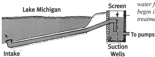
*Six centrifugal pumps lift the water from suction wells to begin its journey through the treatment plant.*
