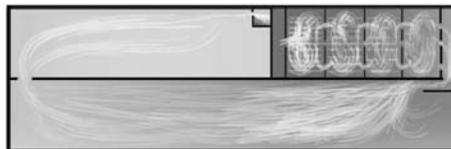
*Water flows through filters which contain a layer of anthracite coal and filter sand, removing the tiniest of particles.*
