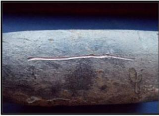
Lead service lines are generally a dull gray color and are very soft. You can identify them easily by carefully scratching with a key. If the pipe is made of lead, the area you've scratched will turn a bright silver color.
